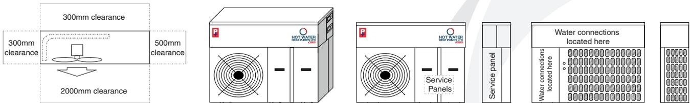
**Note:** 8G R32 Series heat pumps and chillers are not suitable for indoor/plant room installations without air quality monitoring and ventilation due to mild flammability.
